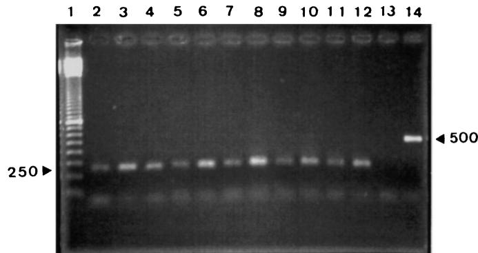
**FIG. 3.** Representative agarose gel (2%) electrophoresis of *EcoRV* restriction digests of amplified regions of the *Pfmdr1* gene containing the codon 1246 polymorphism. Lane 1, 100-bp ladder; lane 2, positive control for 86<sup>Tyr</sup>, 1042<sup>Asp</sup>, or 1246<sup>Tyr</sup>; lanes 3–12, field samples; lane 13, negative control; lane 14, internal control (see text). Band size is indicated in base pairs (bp).
